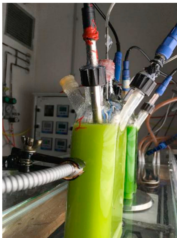
Fig. 2 – Roux-type bottle photobioreactor (1 L working volume) used for the hydrogen experiments with cultures of Chlorella vulgaris strain G-120. The culture behavior was continuously monitored by sensors of pH, DO, and redox potential as well as fluorescence yield by a PAM-2100.
